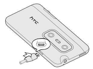
2. Plug in the power adapter to an electrical outlet to start charging the battery.
